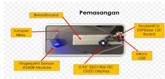
Rajah 5. Pemasangan Don't Skip Class, Ok! : Sistem Kehadiran Kuliah Biometrik
